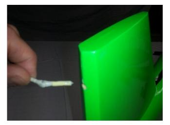
Place a small amount of lubricant on the pin of the hinge and flex the hinge back and forth to coat the pin with lubricant. Lithium grease was used in this model.
