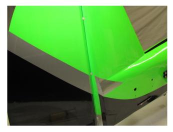
Once all hinges have been installed, clean off excess adhesive. Flex hinge back and forth to help align the hinges in the holes. Rudder hinges have been completed. Note: minimal hinge gap and throw is bevel to bevel. If necessary, increase gap slightly to achieve full control surface throw.
