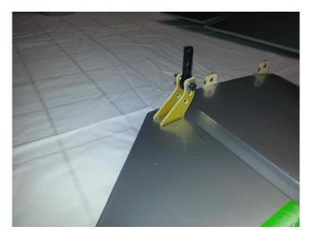
Assemble aileron control horns and tighten bolt. Scuff bottom of control horns (glue area) with coarse sandpaper for better adhesion. Inject epoxy into both control horn slots. Apply additional epoxy to both sides of each control horn. Insert control horns into slots and clean up excess epoxy that oozes out of slots. Elevator control horns have been installed. Note: excess epoxy has not been cleaned off yet.
