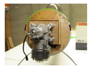
Reinstall engine. This time use thread lock on the mounting bolts.
