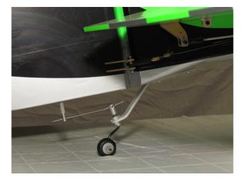
Install rudder servo. Note: spline faces front of airplane. Ball links should be on second to last hole in the arm. Servo arm sweeps toward back of airplane.
