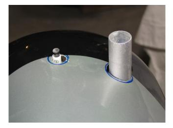
Reinstall cowl. If your template was accurate, muffler and spark plug should line up with holes. Mark final hole sizes allowing for at least 1/8" clearance around muffler. Clearance for spark plug should include ignition cap. Uninstall cowl again.
