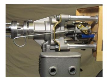
Install muffler with gasket. Use thread lock on bolts.
