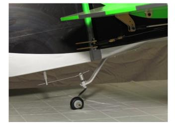
Drill holes for mounting screws.
