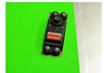
Reinstall aileron servos. Use 12" extension on servo lead. Don't forget to use some sort of restraint on the connector. Restraints are commercially available. Dental floss can be wrapped around the connector and tied 3 or 4 times. Some people like heat shrink tubing. If heat shrink is used, avoid overheating the connector. Install aileron servo. Note: servo spline is closer to the leading edge of the wing.
