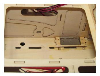
Cut hole in motorbox floor for throttle servo, just in front of wing. Verify location doesn't interfere with wing alignment pin or muffler (if canister). Drill holes in plywood plate for servo mounting screws, then glue into place.
