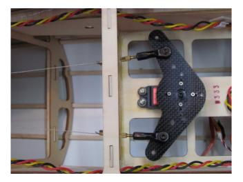
Thread one end of cable onto ball link on rudder horn. Feed cable through fuselage to rudder servo arm. Remove ball link from servo arm. Thread cable end onto ball link. Reattach ball link to servo arm. Install second cable, making sure to cross the cables. Note: getting cables tight enough and centering rudder is a trial and error process. Cables need to be snug, but not "guitar string" tight.
