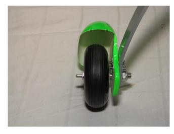
Use wheel collars to center wheel within wheel pant.
