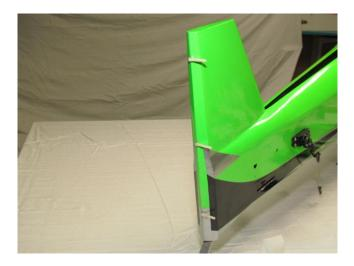
Install all hinges in the flying surface. Make sure all hinges line up the same. If you would like, proceed directly to installing the hinges in the control surface at this time. Inject adhesive into all holes and onto the barbs of all hinges. Make sure all hinges will go in holes. Push rudder into position.
