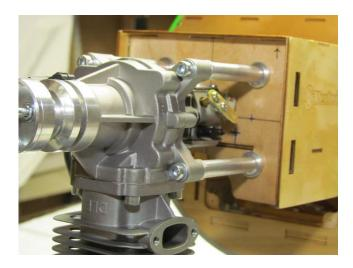
Install standoffs using thread lock on bolts. Note: a 10 mm open end wrench fits on the flats of the standoffs.
