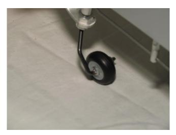
Drill bottom of rudder to accept steering pin. Only insert steering pin about  $\frac{1}{4}$ " into rudder. Install tail wheel and axle. Install steering pushrod, leaving at least  $\frac{1}{2}$ "
