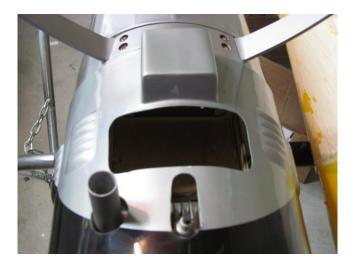
Enlarge holes per revised marks. This time smooth edges, etc. Hole for spark plug includes ignition cap.
