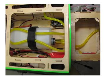
Assemble and install fuel tank. Tank is strapped in with Velcro.
